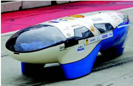
Figure 1 Is that what the car of the future will look like? Agelis ecar built at Royal Institute of Technology, KTH, Stockholm, Sweden, managed to run for 481 km at 1 L of gasoline during Shell Eco Marathon 2010. Critical engine components had antifriction coatings made by Applied Nano Surfaces and a fuel-economy engine oil produced by Elektrion s.a. was used.
