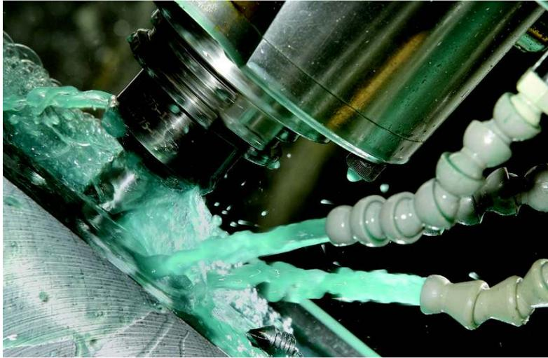
**Figure 1 | Boundary lubricity additives are widely used in metalworking fluid applications. Their selection is particularly critical in high-temperature and pressure applications. (Courtesy of The Lubrizol Corp.)**
